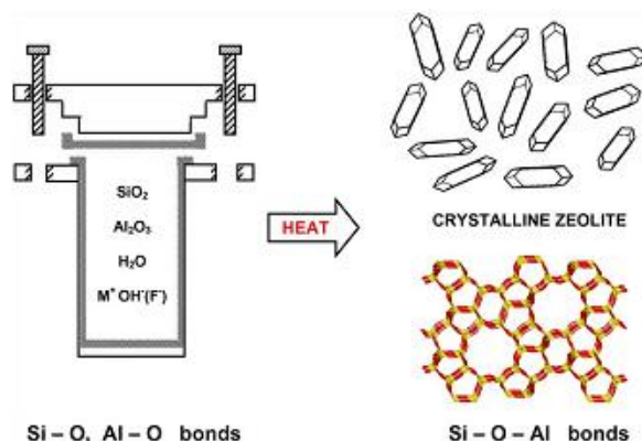
Fig. 1: Hydrothermal Zeolite synthesis (With the use of OSDAs). The starting materials (Si-O-Si and Al-O bonds) are converted by an aqueous mineralizing medium (OH- and/or F-) into the crystalline product (Si-O-Al bonds) whose micro-porosity is defined by the crystal structure
